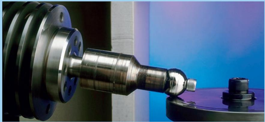
Fig. 6: SKF-WAM 5 tribometer.
