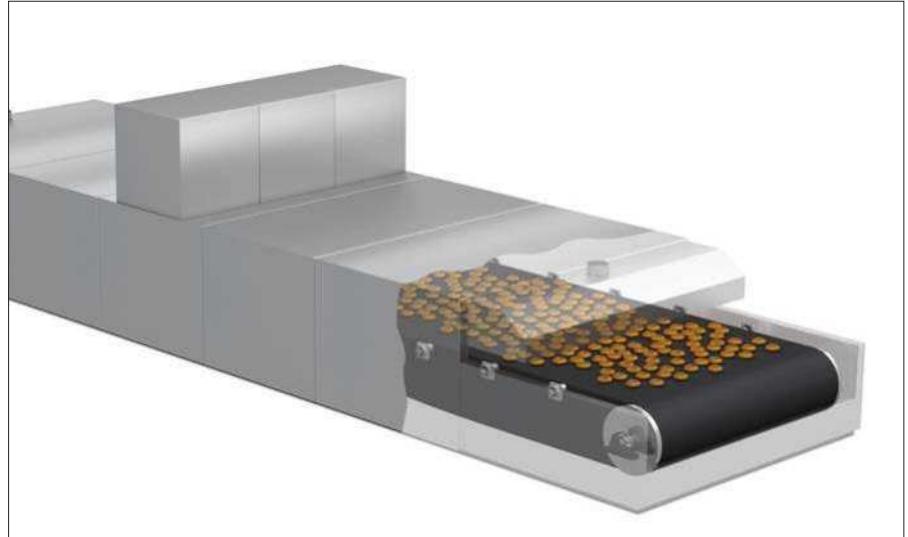
Continuous baking oven using high temperature ball bearing units to support the belt.
