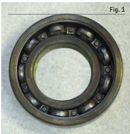
Inadequate lubrication cause wear which can be recognized by noise and excessive play
