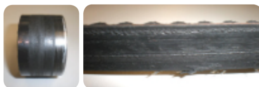
Picture 12: Overheated marks
