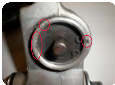
Picture 7: Dent marks on the tensioner body
