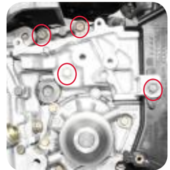
Picture 5: Bolts securing tensioner unit
