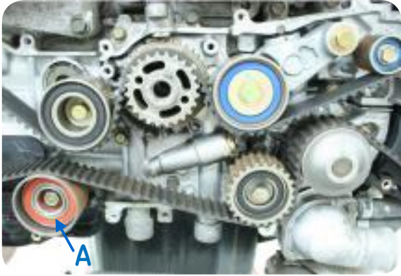
Picture 3: Timing idlers and tensioner locations
