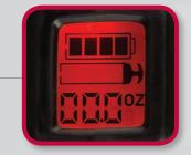
Display flashes red when the gun loses prime or runs out of grease
