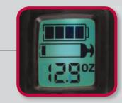
Grease level flashes when low grease condition occurs
