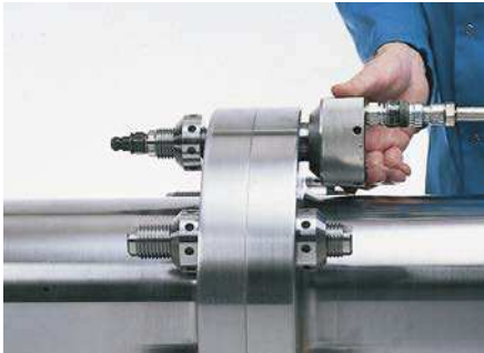
7. As an alternative, the bolt can be pulled out from the sleeve, with the tensioner mounted on the opposite side.
