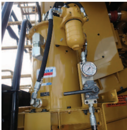
The mechanically operated, easy-to-install overflow prevention system is compatible with any pump using a Lincoln FlowMaster reservoir.
