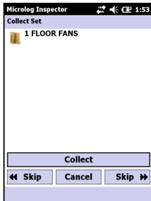
If the setting is configured to “Off”, the Sets will still display in the ROUTEs screen (left) but the “Collect Set” screen (right) will be skipped and the user will proceed to the first Machine under the set.
