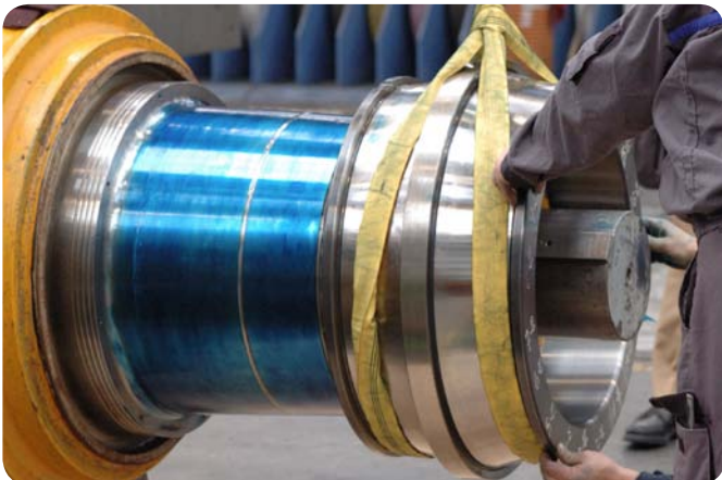
Fig. 6 An inner ring ready to be slammed against a Prussian blue coated tapered seat.
