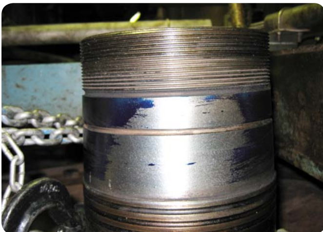
Fig. 4 The absence of Prussian blue indicates no contact between the ring and the journal.
