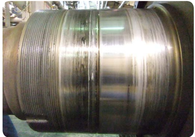
Fig. 1 Fretting corrosion and smearing on a press roll journal, but why is it only on the left hand side?
