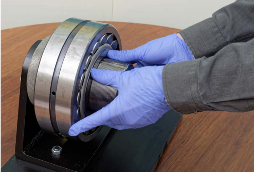
Fig. 4 Place the bearing on its tapered seat
