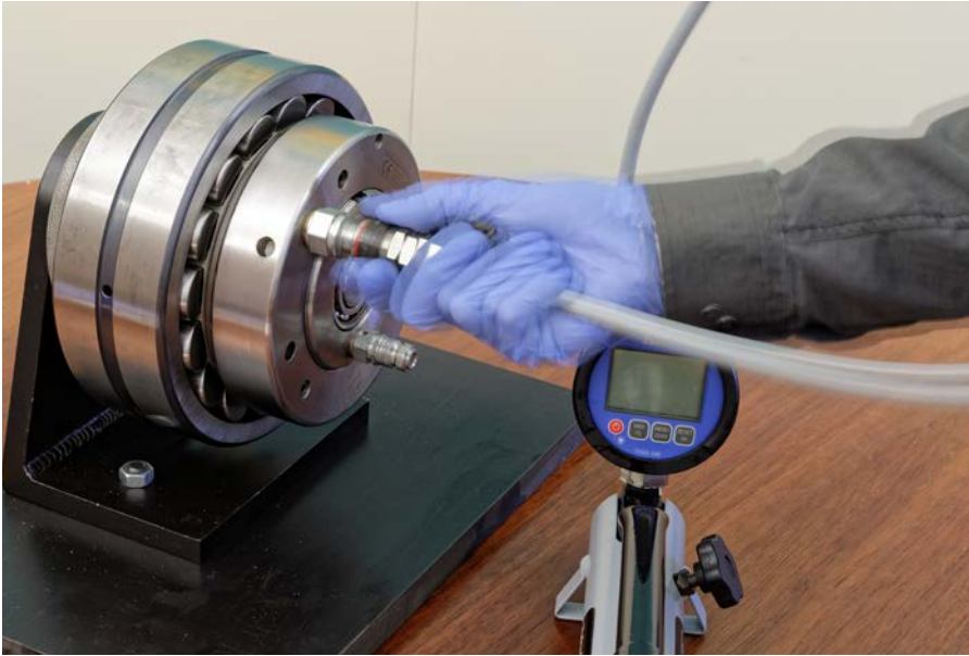
Fig. 7 Connect the pump to the hydraulic nut
