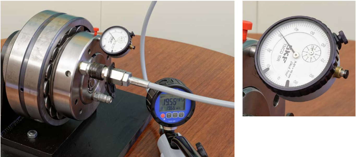
Fig. 14 Final axial position is reached
