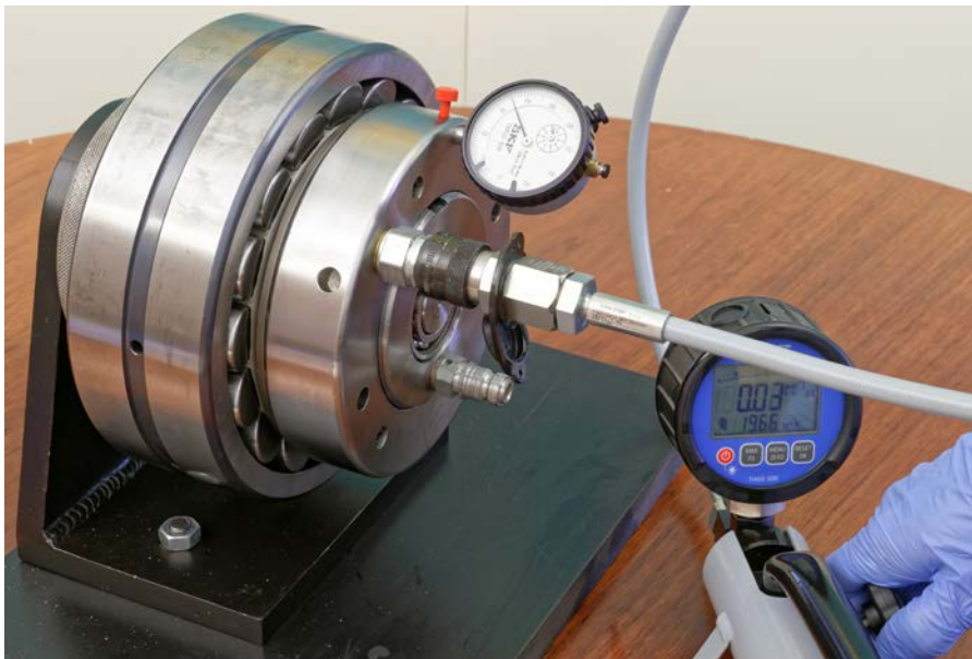
Fig. 16 The dial indicator needle moves backwards when the oil pressure is released
