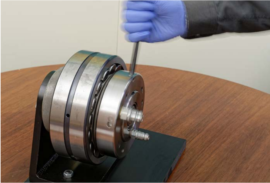
Fig. 6 Mount the hydraulic nut and tighten it by hand
