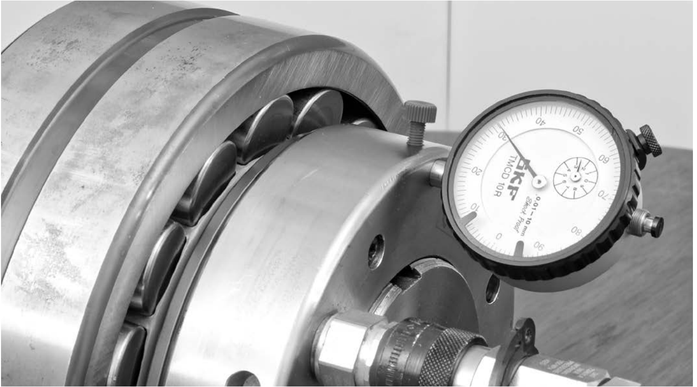
The main tools for the SKF Drive-up Method: A dial indicator and a hydraulic nut
