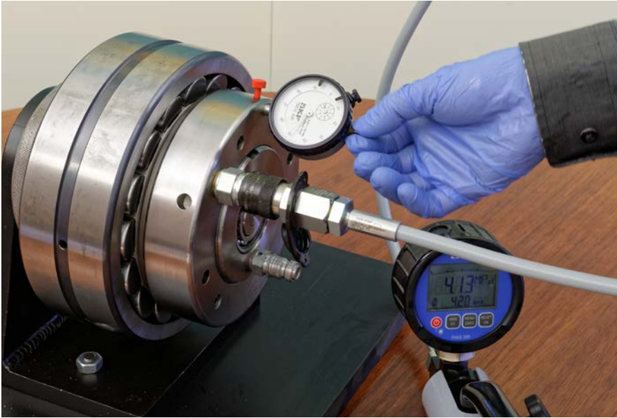
Fig. 11 Place the dial indicator in the hydraulic nut so that it can follow the axial displacement of the bearing until the final drive up value is reached
