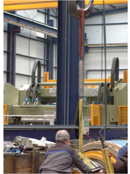
Fig. 5 Using a spring for easier handling during mounting or Prussian blue tests
