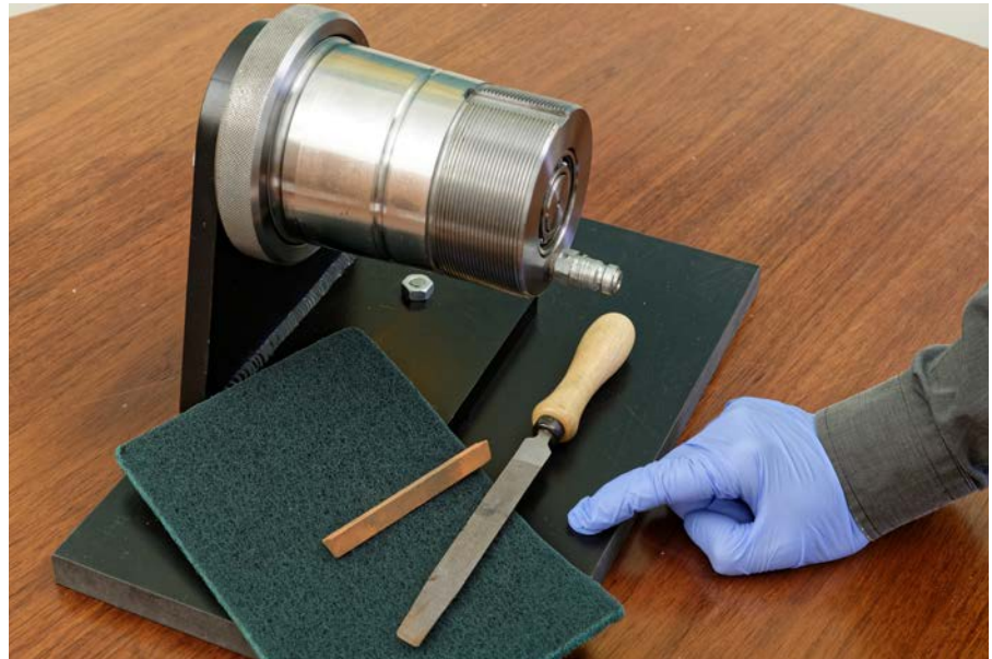
Fig. 2 Tools: scrub pad, steel file, honing stone and a finger
