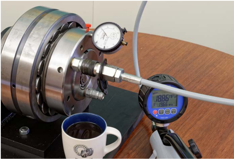
Fig. 15 When the final drive-up value is reached, take a coffee break
