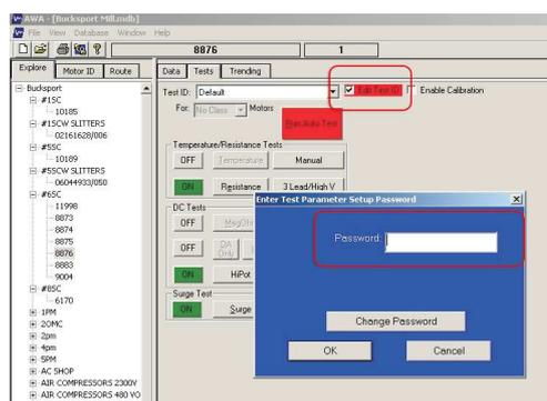
Figure 7. Setting a password within the Tests tab.
