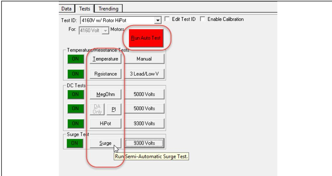
**Figure 19.** Controls used to run automatic and semi-automatic testing.
