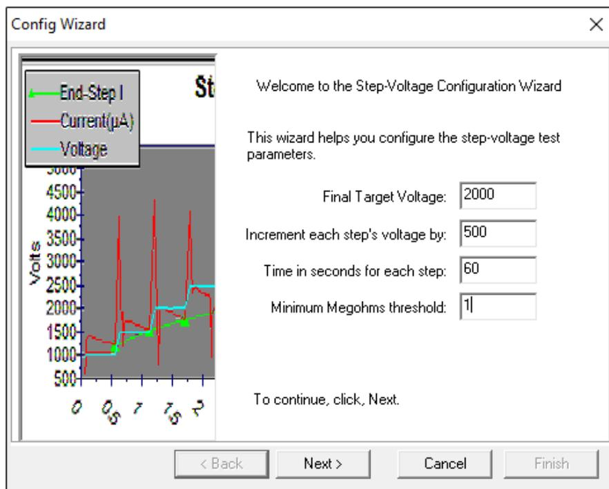
Figure 15. Step-Voltage Configuration Wizard; setting voltage parameters.
