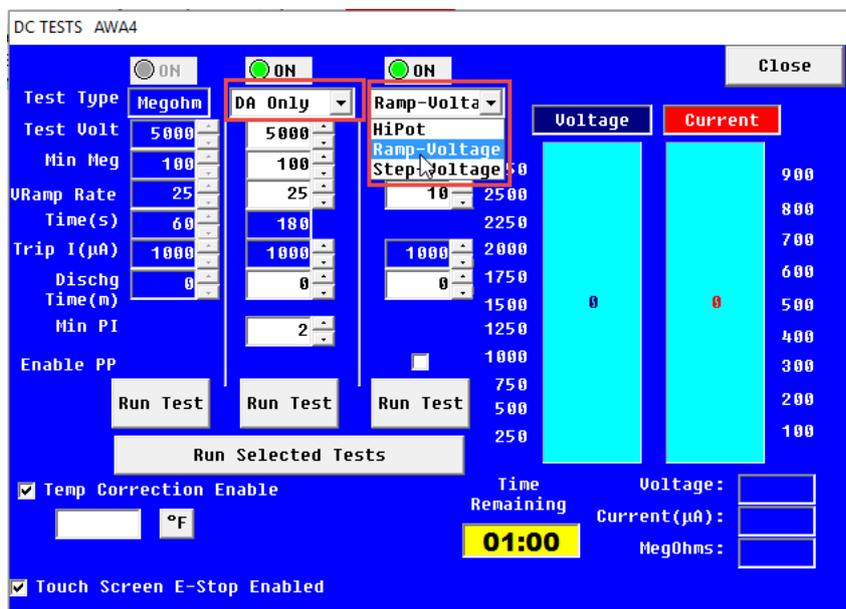
**Figure 10.** Selecting test parameters from the DC Tests Setup screen.
