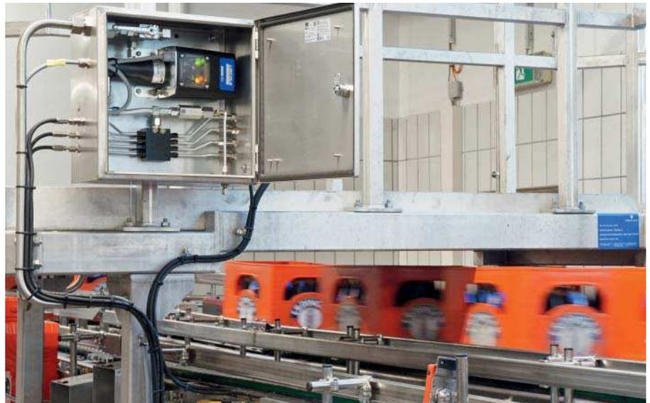
View into a section cabinet with EDL1, progressive feeder and stopcock to the main line
