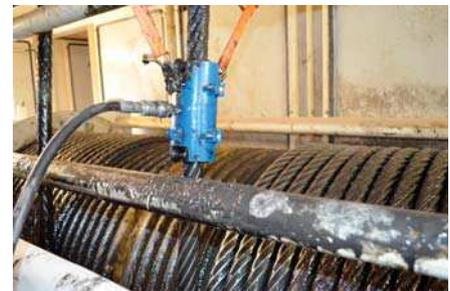
*The lubricator is applied intermittently on this wire rope to provide lubrication, which means that it can be used consecutively for many different ropes.*
