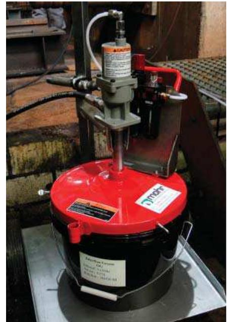
The lubrication system applies the correct amount of lubricant and distributes it evenly, thereby preventing over-lubrication.
