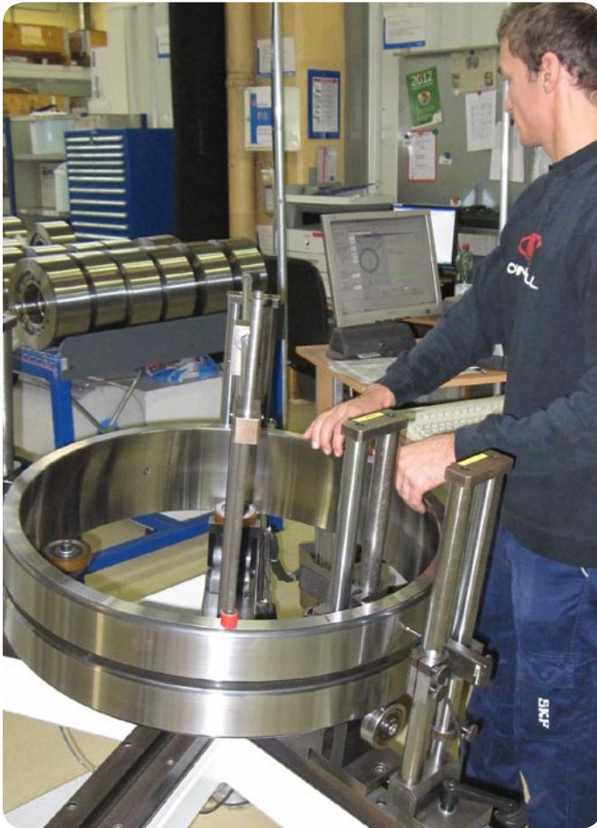
Fig. 11 Ring ovality and wall thickness variation measurement
