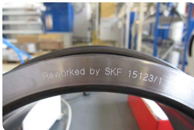
Fig. 4 Traceability number indicating the centre of the new load zone. Here it is marked on the bearing inner ring since it is for a deflection compensating roll where the outer ring rotates with the cylinder.
