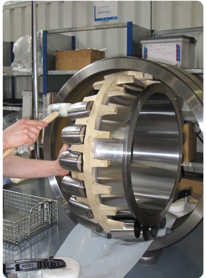
Fig. 12 Special care is taken during assembly to ensure that rollers do not mark the raceway.
