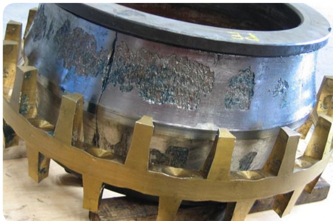
Fig. 5 Heavy spalling means that this ring needs to be scrapped
