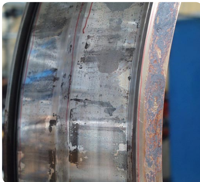
Fig. 6 The corroded inner ring of a deflection compensating roll
