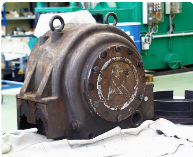
Fig. 13 Rocker housing before modification.
