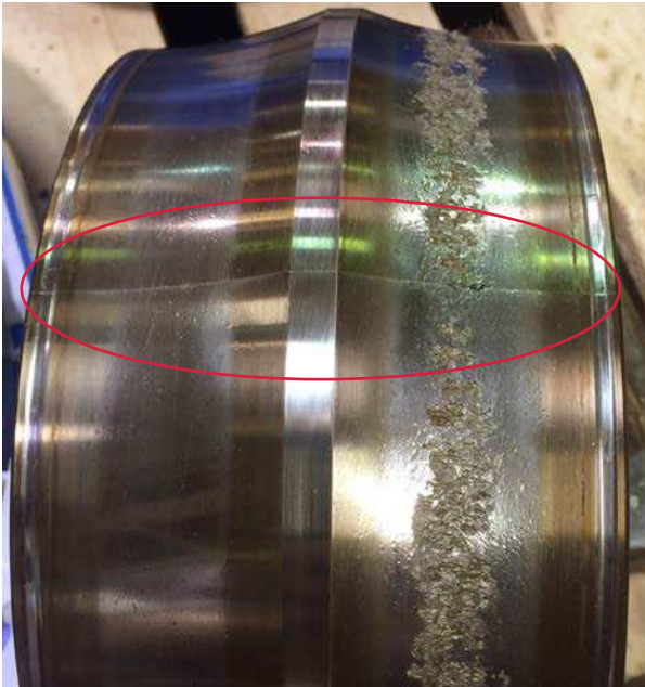
Fig. 16: Damaged bearing inner and outer rings
