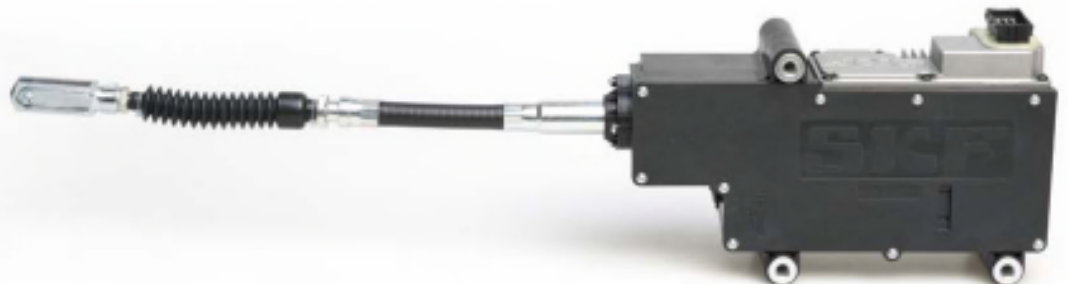
SKF Electronic Parking Brake with customised Bowden cable
