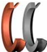
V-ring seals from SKF offer an easy-to-install solution for rotating shaft applications, including use as a secondary seal in highly contaminated environments. They can be stretched and, depending on the size, pushed over other components like flanges, pulleys or even housings.
