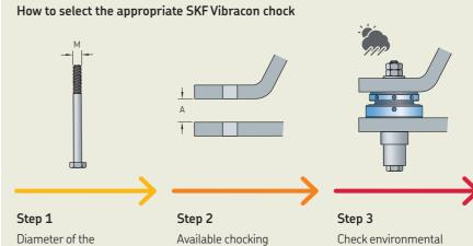
Diameter of the foundation bolt (M)
