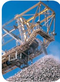
Operating conditions in vibrating screens can quickly overheat and destroy conventional bearings. The result is frequent shutdowns to rebuild equipment – contributing to high maintenance costs.
