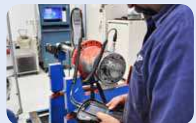
Testing verifies speed, vibration, temperature and critical runouts
