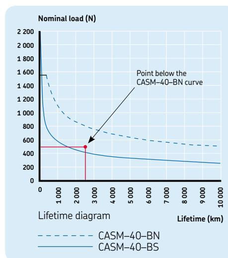
In this example, the CASM-40-BN is the smallest possible linear unit.
