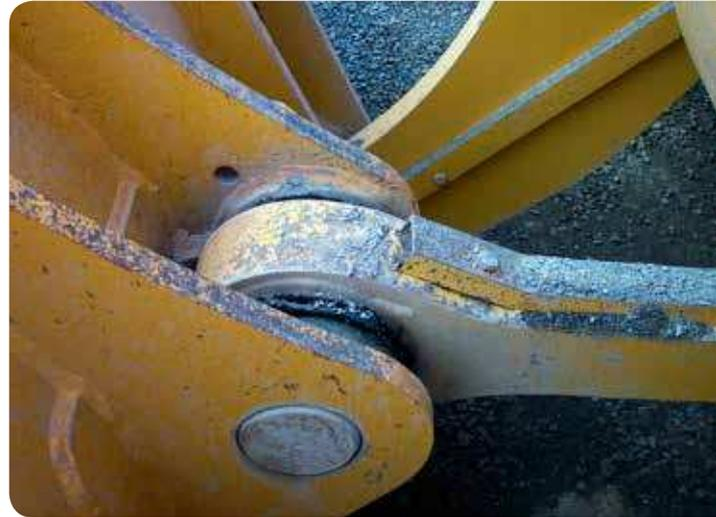
Automatic lubrication systems supply the correct amount of grease at the best time to lubricate – while the bearing is in motion. Frequent lubrication maintains the proper lubricant film to reduce wear, as well as purges the pins and bushings of contaminants.
