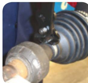
using special pliers with an integrated hold-down device; this prevents the unintentional opening of the clamps after tightening.
