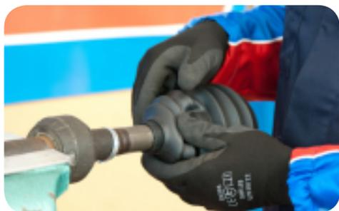
2. Locate the CV-joint on to the spline on the end of the shaft, then tap the
