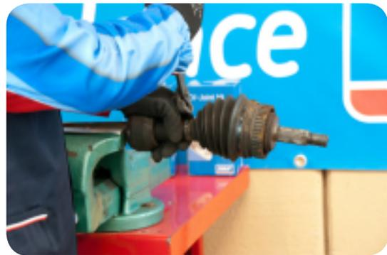
4. In order to clearly see the snap ring, remove the grease from around the base of the shaft. Then with suitable pliers, hold the snap ring open. The CV-joint is then ready to be removed from the shaft.
