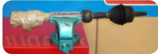
3. Remove both the inner and outer clips. Then, cut the boot and remove it.
