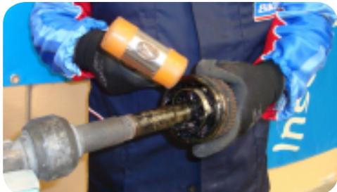
3. Slide the boot into position ready for mounting and fill with all of the supplied grease.
