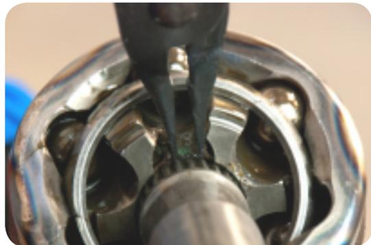
5. Hold the CV-joint and pull it off the shaft. Lightly tapping with a hammer may help.
