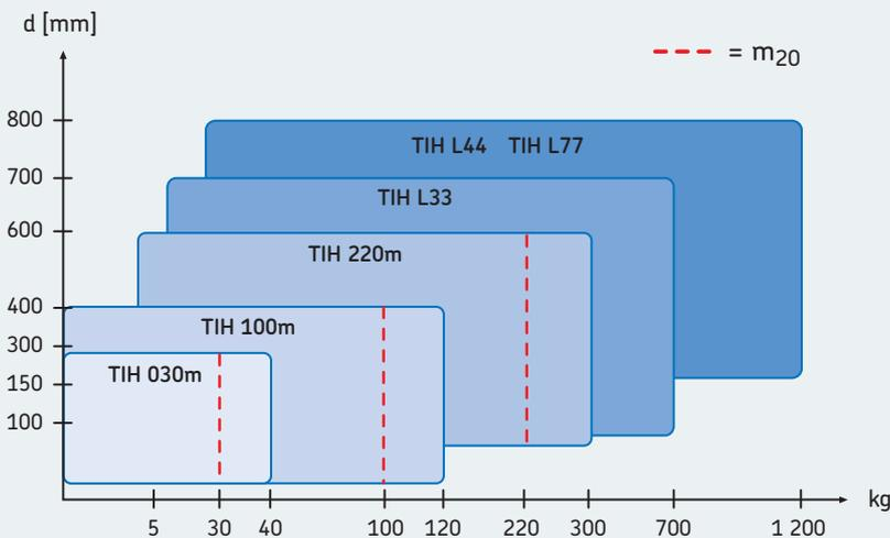
The comprehensive range of SKF induction heaters is suitable for most bearing heating applications. The chart gives general information on choosing an induction heater for bearing heating applications<sup>1)</sup>.
