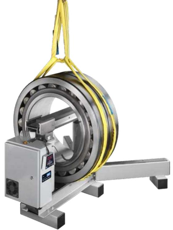
Large induction heater with a 700 kg bearing heating capacity
