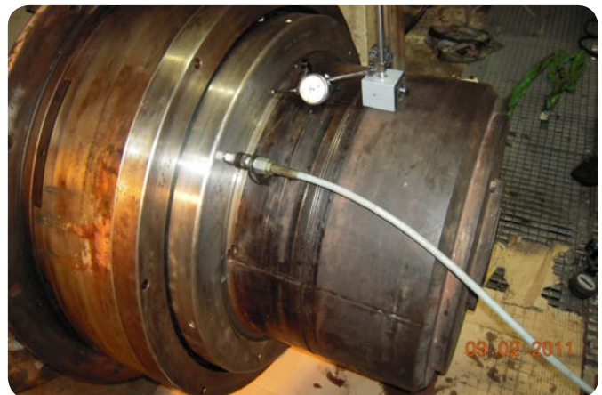
Fig. 1 Axial displacement of the adapter sleeve
