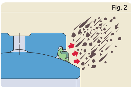
A steel insert protects the seal lips from damage
