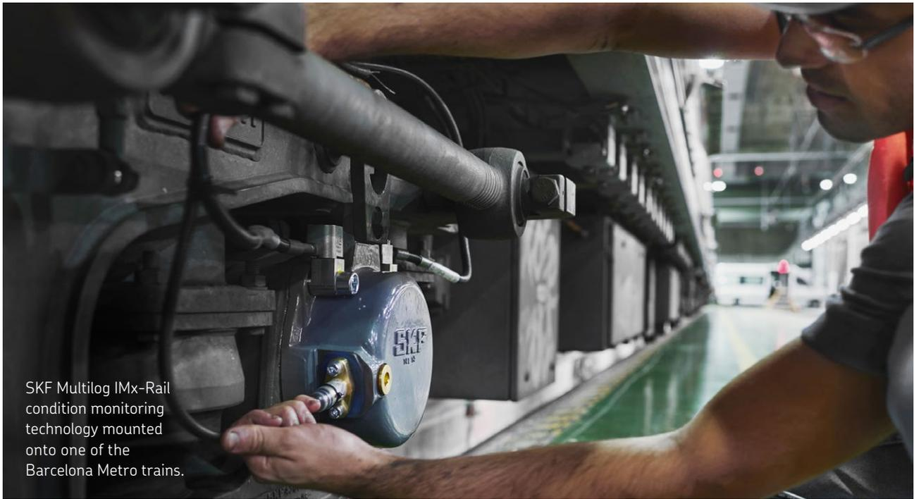
SKF Multilog IMx-Rail condition monitoring technology mounted onto one of the Barcelona Metro trains.
