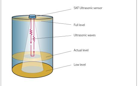
The SKF Ultrasonic sensor was developed to improve fill-level monitoring on SKF- and Lincoln-branded pumps and reservoirs with lubricant capacities in excess of five litre. Suitable for oil and grease applications, the sensor provides continuous level messages for optimum operation. Maintaining the appropriate amount of
