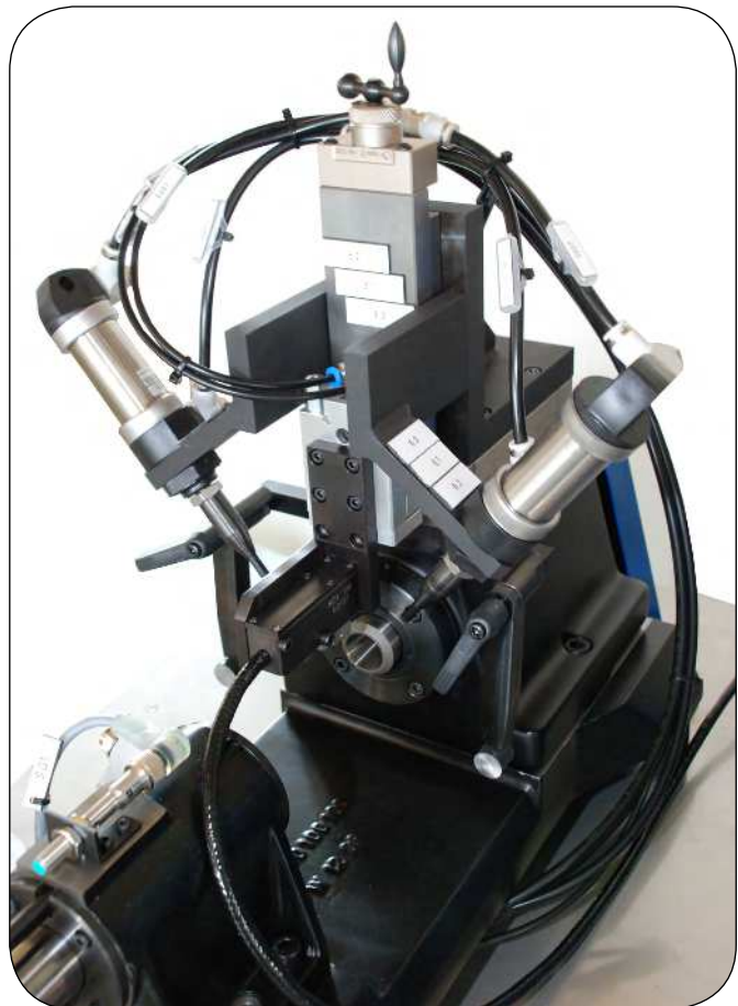
MVH 90E mechanics with axial load and radial load
