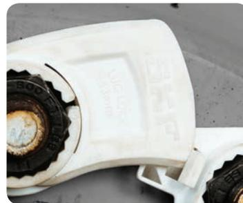
*As the wheel nut loosens, the lug lock rotates and provides an easily visible indication that the wheel nut is in need of re-torque.*
