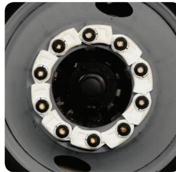
*When the lug locks are installed properly, they create a consistent look indicating all wheel nuts are secure.*
