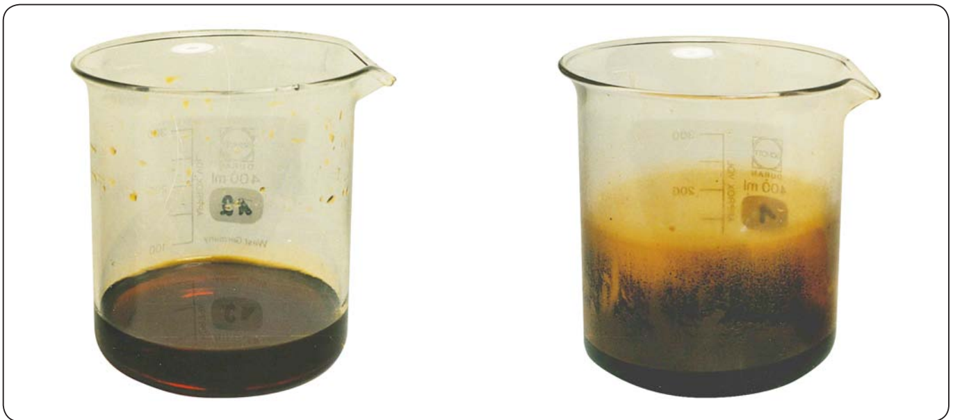
Fig. 7 Two different mineral oils after 8 weeks at 120 °C (248 °F). The oil on the left is suitable while the one on the right is unsuitable.
