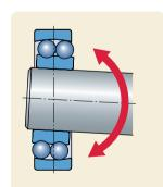
SKF self-aligning ball bearings accommodate typical misalignment conditions.
