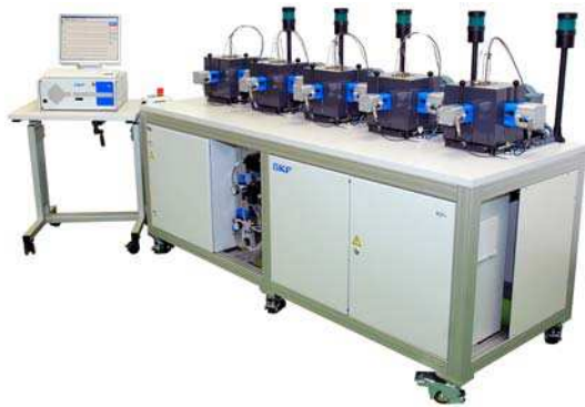
Figure 2. The ROF+ set-up: five units, where each unit contains two test bearings.
