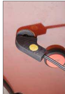
Fig.15 – Place the magnetic probe on a metallic surface, such as a bolt on the EAZ
