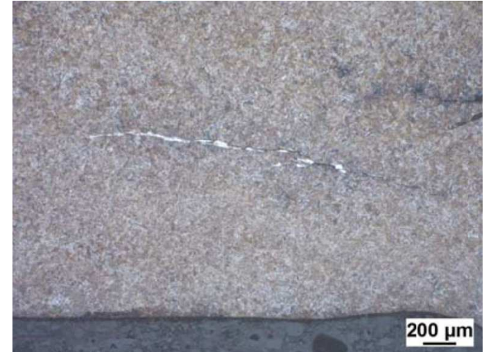
White etching crack in large TRB rolling contact fatigue test
