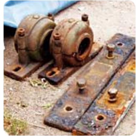
*The old bearing housings and fixing plate*
