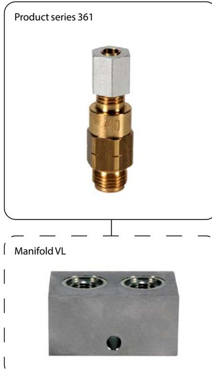
The distributor body of the design for oil is made of brass. The design for oil/fluid grease has a distributor body made of steel (galvanized, Cr6-free). The seal of the internal thread for mounting the single-port single-line distributor in a manifold is available in a flat washer design.
