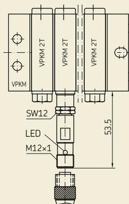
Sectional metering device VPK with visual cycle indicator
