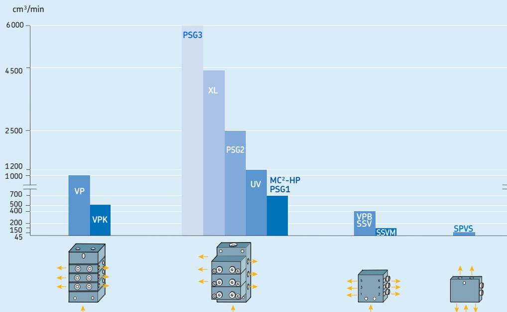
The maximum recommended flow rate values relate to lubricating oil at the highest selectable piston-stroke volume.
