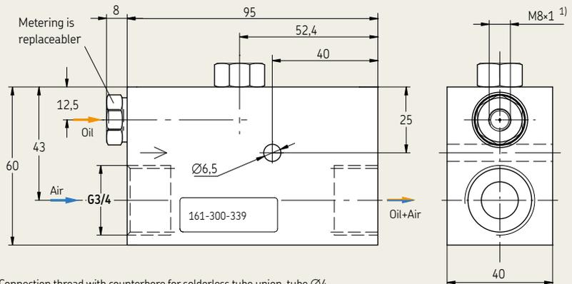
1) Connection thread with counterbore for solderless tube union, tube Ø4.
