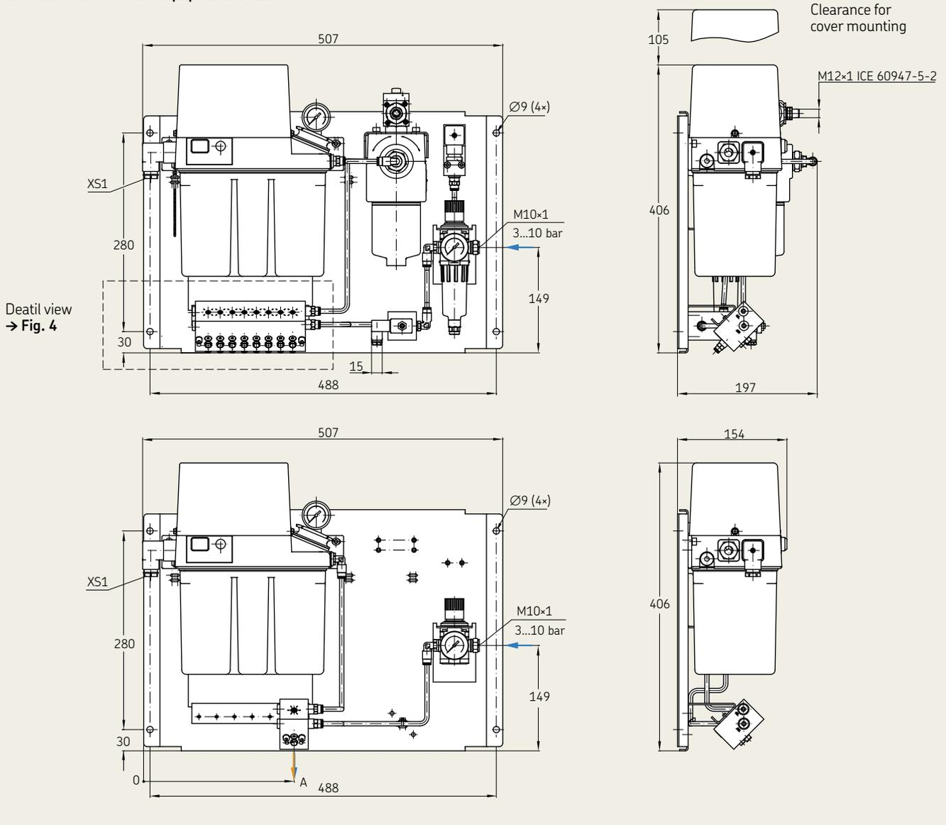
Dimensions of oil+air mixing valve with metering
