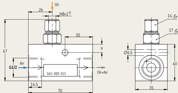
1) Connection thread with counterbore for solderless tube union, tube Ø4.
