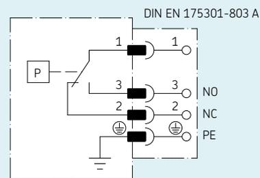
Contact position shown: Switch depressurized
