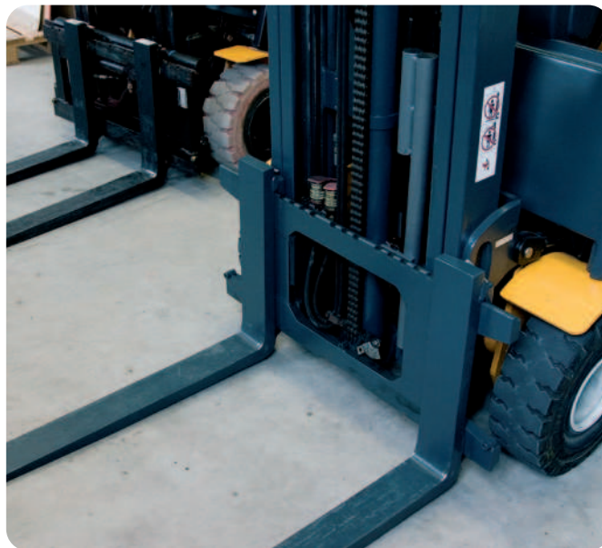
SKF Leaf Chains used for lifting in a forklift mast
